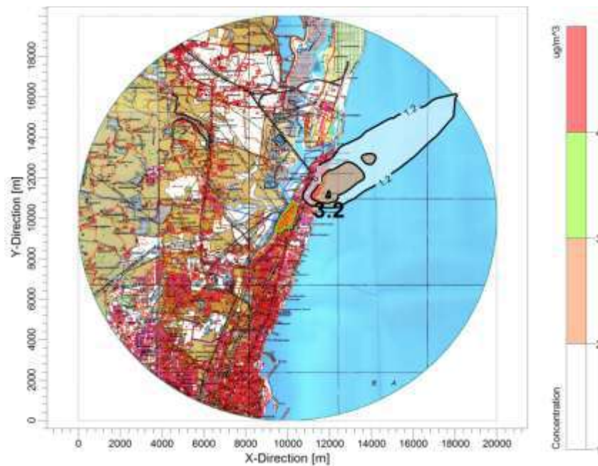
Figure 4.5: Predicted 24-hourly average GLCs of NO x (µg/m 3 ) for 1x660MW (260 g/Gj)
