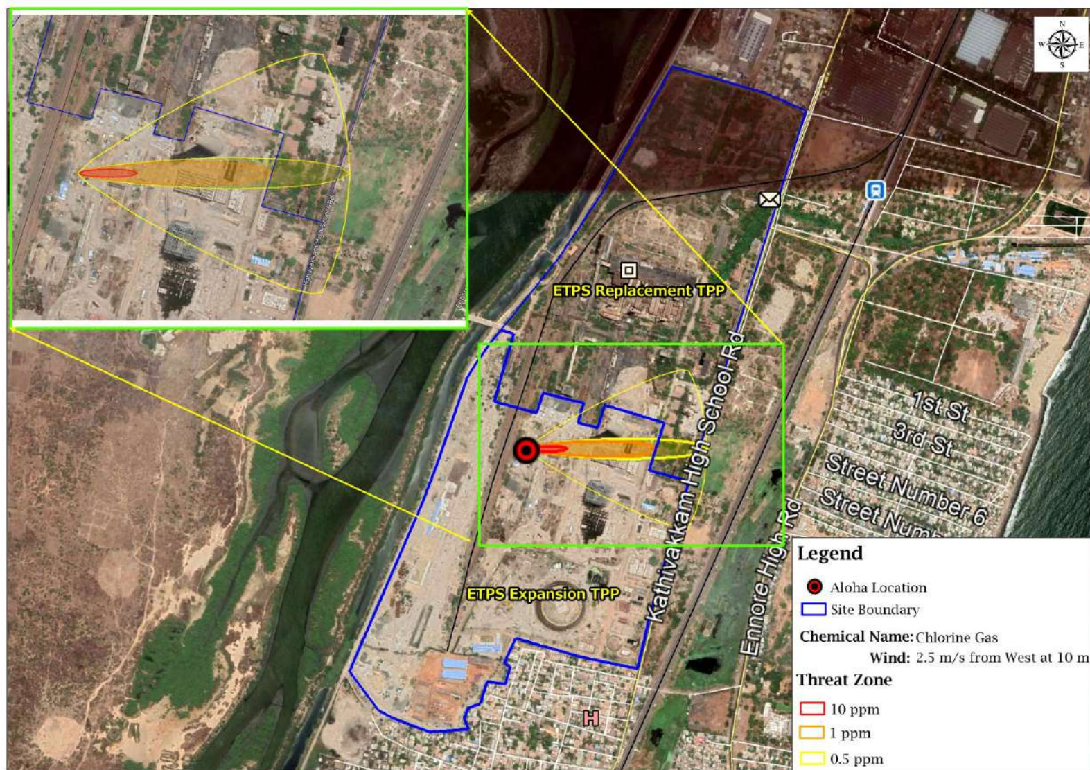
Figure 7.5: ALOHA risk plotting for chlorine gas
