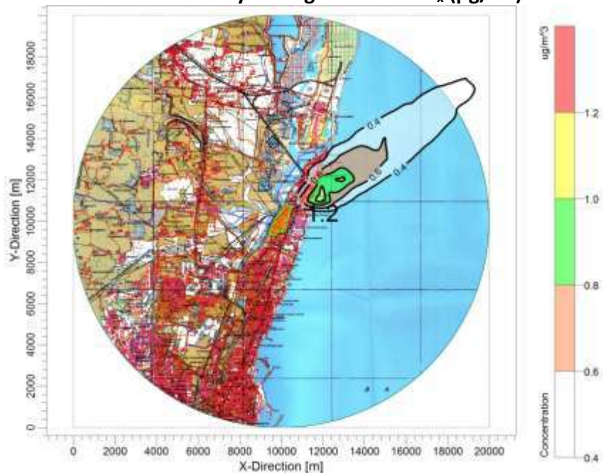
Figure 4.4: Predicted 24-hourly average GLCs of NO x (µg/m 3 ) for 1x660MW
